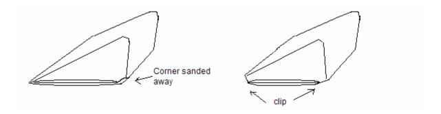
**Edges are still leaking:** If the edges are too thick, remove the head and take some fine sandpaper and thin the edges so that they close properly.
