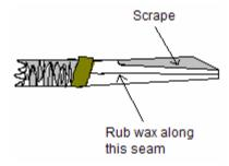
**Check the corners** of the reed lips to see if they have been sanded off. If they have and it is only sleight, then the problem can be solved by clipping the corners of the reed at an angle.
