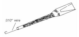
**New staple:** If you have come this far it is time to try a new staple with a smaller inside diameter. Wrap string around the head, remove the binding, insert the new staple and re-bind with fresh binding and go through the above steps again. Keep this up until you either solve the problem or purchase/make another reed.
